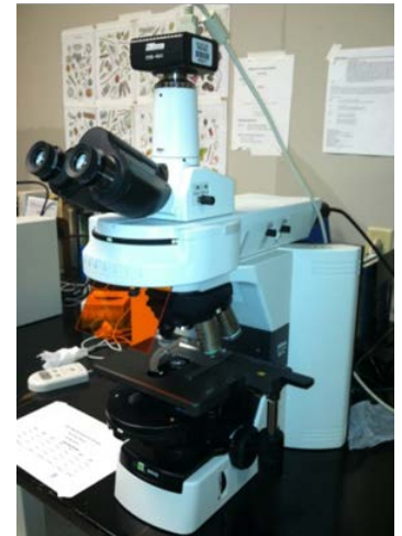
The photos shown here are (above) one of the fluorescing microscopes utilized by IDEM staff to identify and enumerate / count algal cells, and (below)
