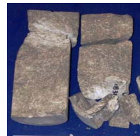
Louisville Tunnel Project 1831-10-5629 Boring 91 Sample 6 (Run 10 Box 4) 64.4' (Unconfined)
