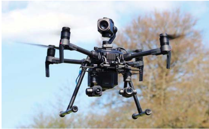
Figure 10.3 A drone equipped with cameras for leak surveys. (Source: Bath Echo)
