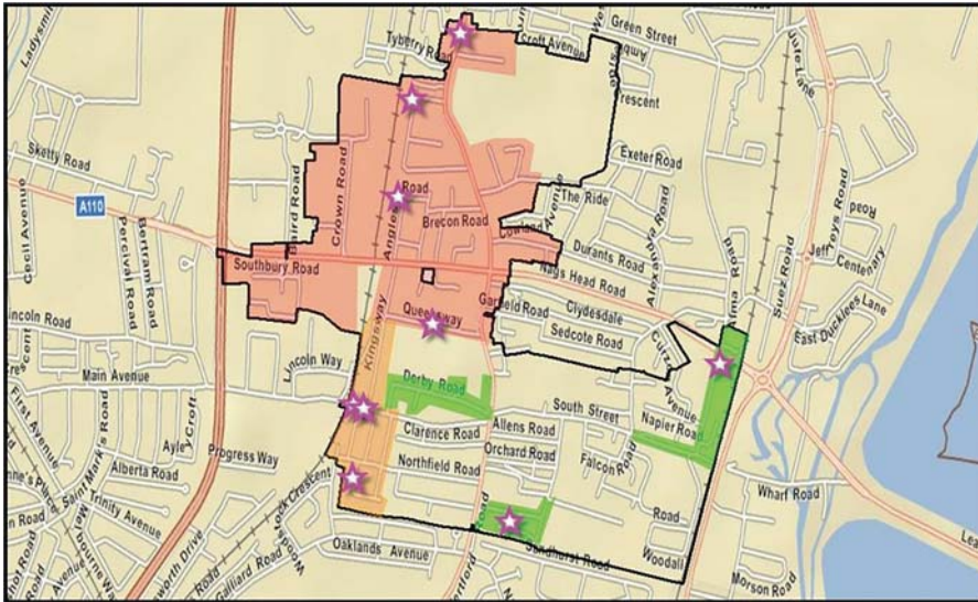
Figure 17.4.2 Confirmed leaks identified by “Burstfinder”. (Source: GL Industrial Services)
