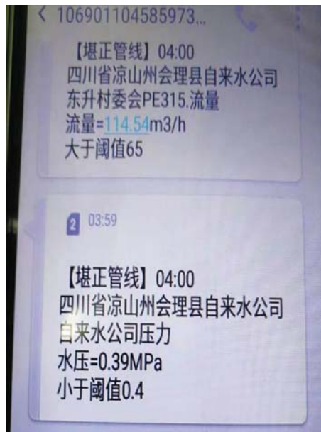
Figure 17.9.5 SMS alarm. (Source: Yunnan Kan Zheng Water Loss Control & Engineering Co., Ltd)
