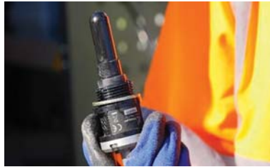
Figure 17.10.3 Enigma3hyQ logger. (Source: Anglian Water)
