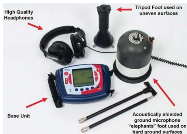
Figure 7.2 Components of electronic amplified listening device. (Source: Halma Water Management)
