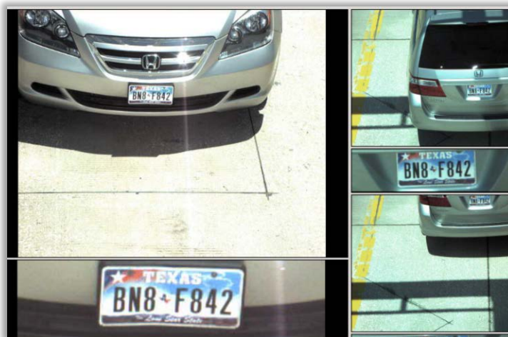
Figure 2-8: Example of Images Captured by Toll Zone ETCS Cameras
