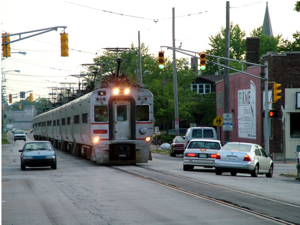
Figure 5-10 – A South Shore Line train runs along the embedded street-running in Michigan City
